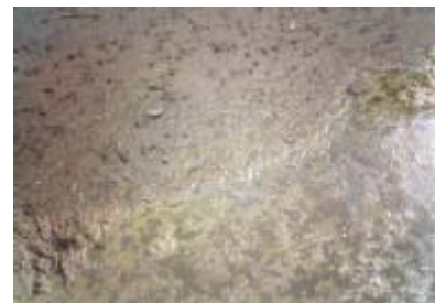
Scum and crust formation 1 week after application of Advetec 900.
